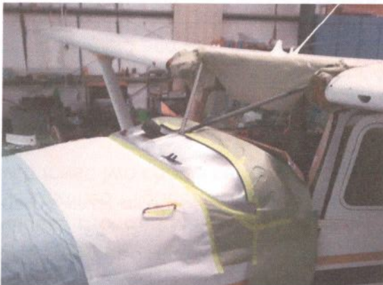
Ready to repaint glareshield & brace
